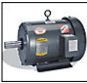
Motors built for applications requiring F-2 mounting are available from stock in 1/2 HP through 60 HP. These motors are manufactured in both TEFC and Open Drip Proof construction in NEMA frames from 56 to and including 364T. Many of the ratings are Class "F" insulated with 1.15 Service Factor that operate within Class "B" temperature limits. The motors are stocked in both Standard High Efficiency and Premium Efficiency designs.
