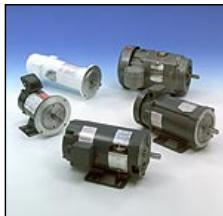
Boston Gear offers a wide range of ODP (open drip proof) AC motors, including brake motors. These motors are offered in C-Face models for mounting to our enclosed gear drives, and they are available in 1/6 - 20 HP and cover voltage ranges from 115 VAC to 460 VAC. These motors are ideally suited for use in environments where dust or other particles can't enter the louvers through the bottom.
