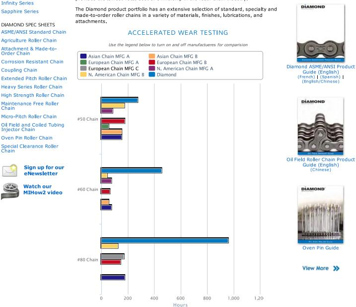
\* #50 Test conditions: 1172 RPMs, 91 lbs. of tension, 3.5 chain horsepower and 21T X 21T sprockets.
